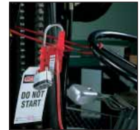
Immobilize large or cumbersome devices, such as forklifts
