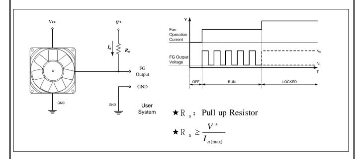
■ Electrical Characteristics: at Ta=25°C, Vcc=12V
