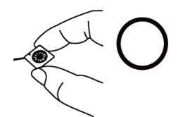
Don't pull fan with lead wires.
