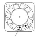
Note: The glues on the impeller is for impeller balance.
