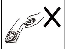
Don't cut the fan or lead wires
