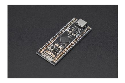
This compact STM32F411 development board can be well embedded in your projects. Featuring the STM32F411CEU6, this chip has 512KB of ROM, 128KB of SRAM and runs at 100MHz. There is a spot on the bottom for SOIC flash memory, which allows you to solder SPI flash memory to give yourself more space for data logging or file storage.
