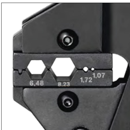
Replaceable crimp insert
