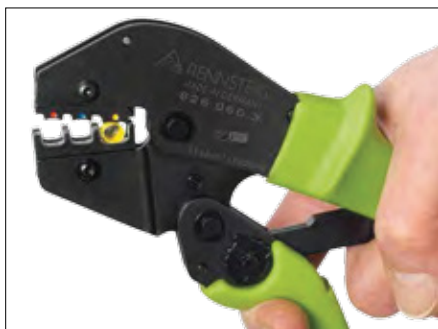
Locate the contact with low force
