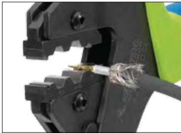
Inner conductor crimp
