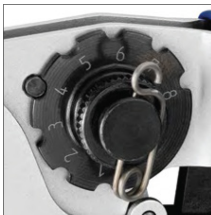
Crimp indent adjustment by 8-position MIL-type selector
