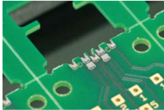
PCB with solder paste and pre-form
