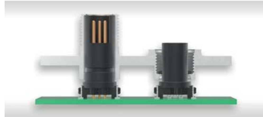
Standard variants integrated in customer housing 13 mm die-cast
