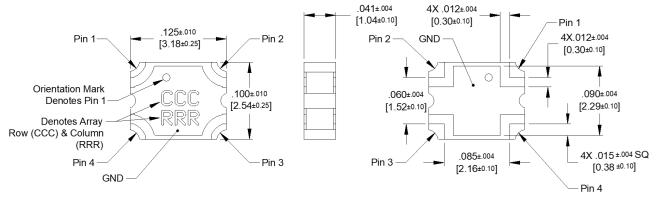
Dimensions are in Inches [Millimeters] X4C40K1-15S Mechanical Outline
