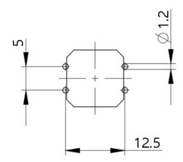
PCB hole pattern component side
