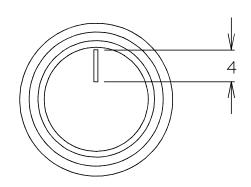
Base Diameter: 19.1mm Overall height: 16mm Shaft depth: 14mm
