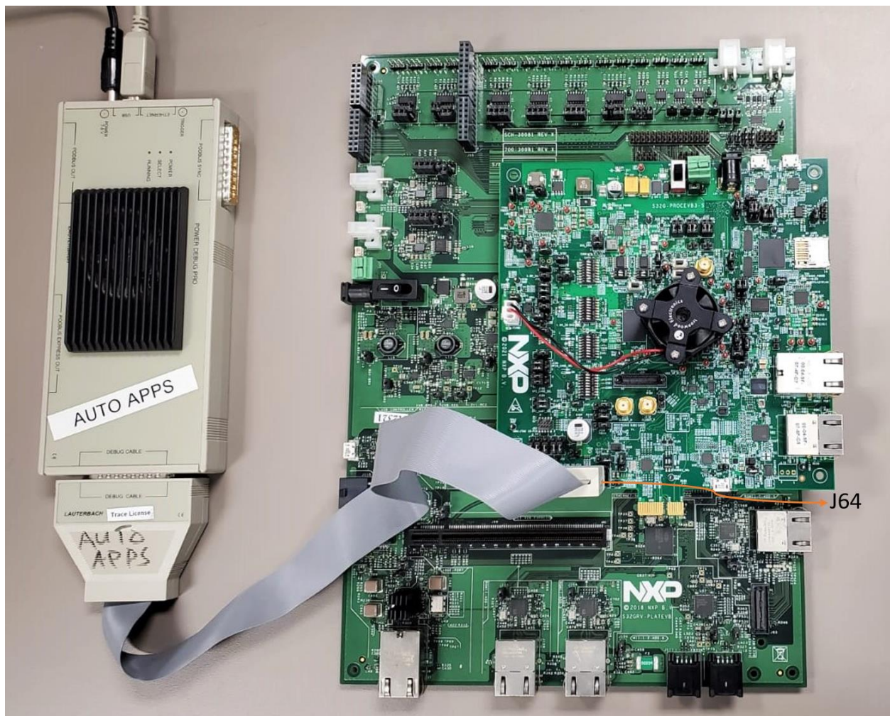
Figure 10. Connecting 20-pin Lauterbach cable on S32G-PROCEVB3-S
