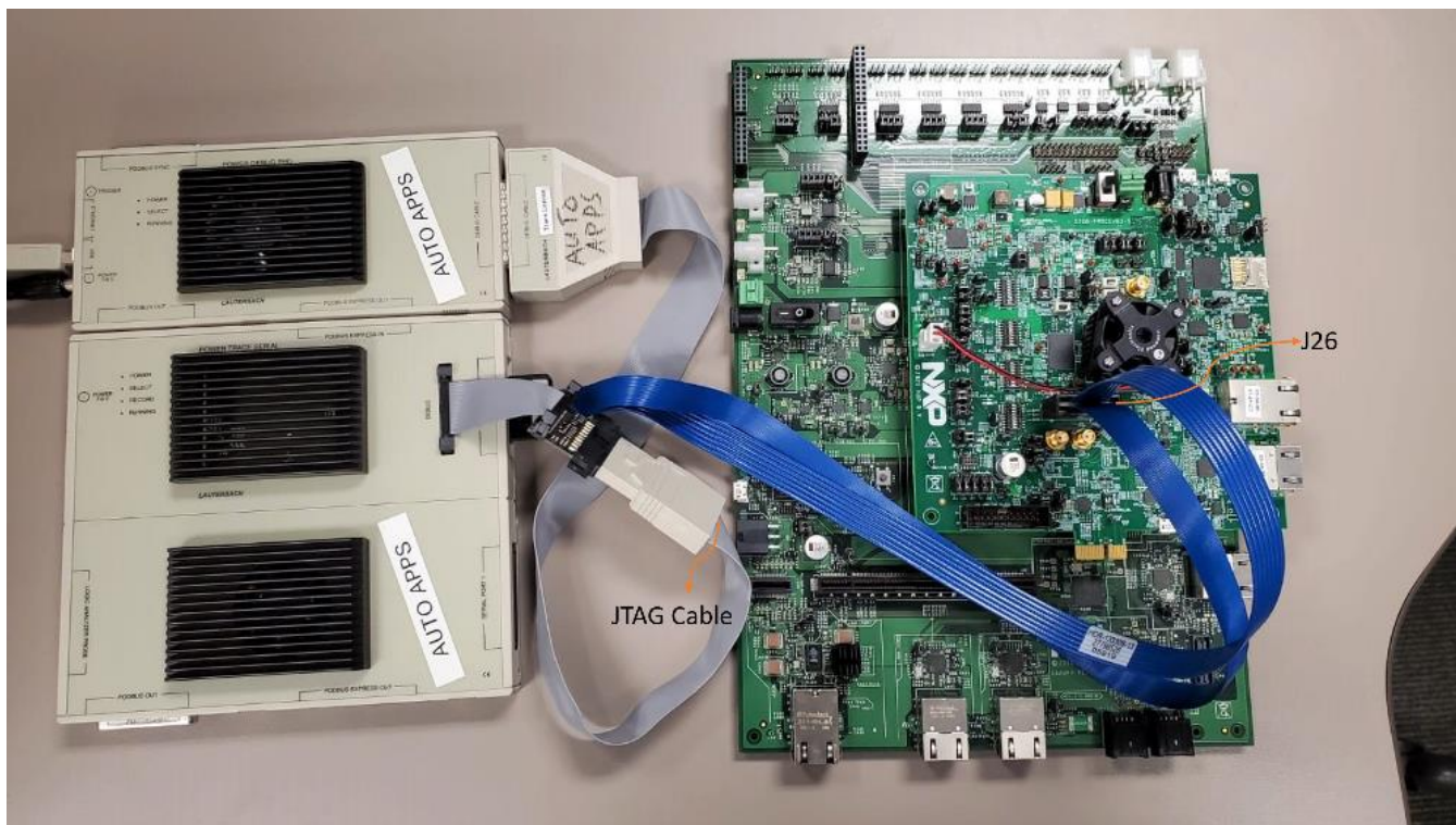
Figure 15. Aurora Port setup 1 with only ATP cable connected to S32G-VNP-EVB3
