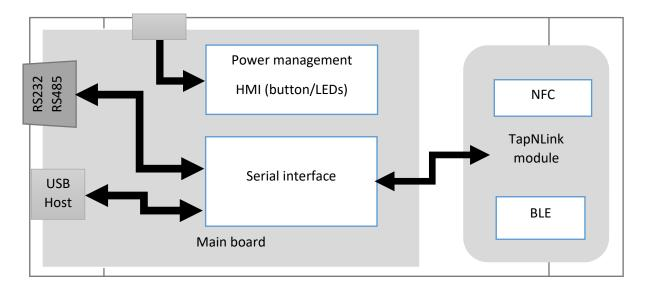
The TapNPass embeds a standard TapNLink module. This module manages radio communication, while serial communication is performed by the main board.
