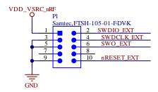
Figure 10: SWD BL5340PA development board schematic
