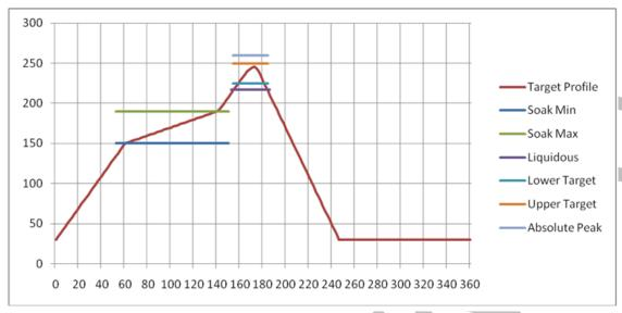
Figure 21: Recommended reflow temperature
