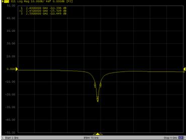
Figure 11: 453-00068 on-board PCB antenna performance (Antenna Gain and S11 – whilst 453-00068 module sitting on Devboard 453-00068-K1)
