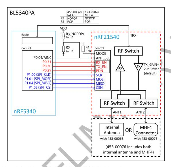
Figure 12: Block Diagram of Front End Module (FEM) nRF21540 Control
