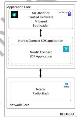
Figure 7: Functional SW block diagram for BL5340PA series BLE module
