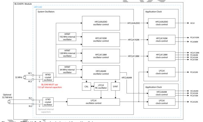
Figure 4: nRF5340 SoC clocks (adapted from Nordic)
