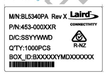
Figure 19: Antistatic bag and box labels
