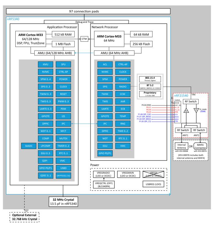
Figure 1: BL5340PA HW block diagram
