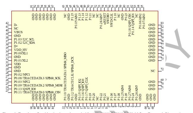
Figure 2: Top view - Combined schematic symbol for 453-00068 BL5340PA Multi-Core/Protocol -Bluetooth +802.15.4+NFC Module (Nordic nRF5340) - Integrated Antenna and schematic symbol for 453-00076 BL5340PA Multi-Core/Protocol -Bluetooth +802.15.4+NFC Module (Nordic nRF5340) -MHF4 RF connector
