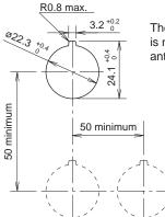
The 3.2-mm-wide key recess is necessary when the anti-rotation ring is used.
