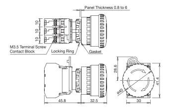
Note: When pressed, the button is locked in the depressed position, and is reset when either pulled or turned clockwise.
