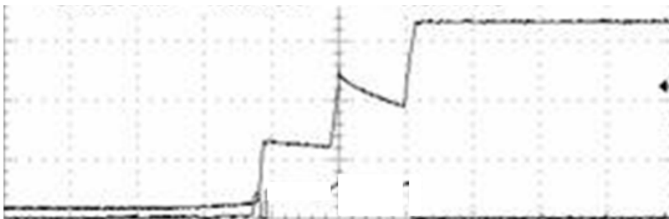
Figure 24. Supply Voltage Drop
