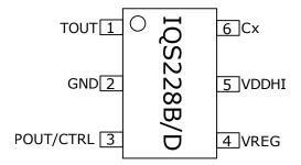
Figure 2.1: IQS228B/D TSOT23-6 Pin-out
