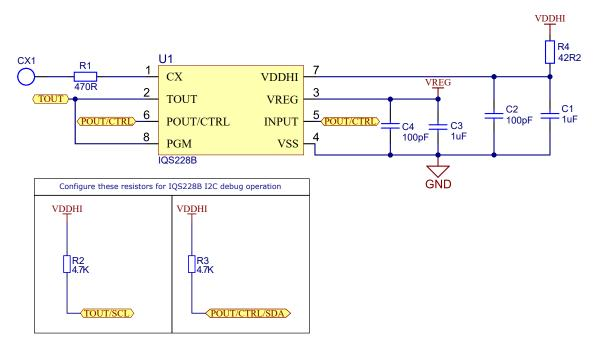
Figure 3.2: Typical application reference schematic of IQS228B WLCSP-8 Package. 100 pF capacitors are optional for added RF immunity. Place all decoupling capacitors (on VDDHI and VREG) as close to the IC as possible.
