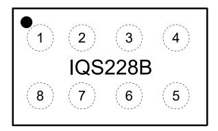
Figure 2.2: IQS228B WLCSP-8 Pin-out
