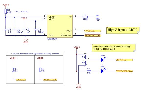
Figure 3.1: Typical application reference schematic of IQS228B/D. 100 pF capacitors are optional for added RF immunity. Place all decoupling capacitors (on VDDHI and VREG) as close to the IC as possible.
