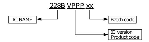
Figure 13.3: Top Marking of IQS228B WLCSP Package
