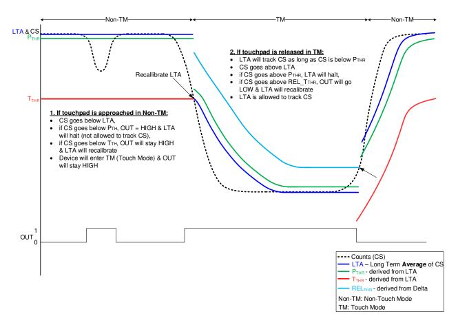
Figure 6.1: DYCAL Operation (Self Capacitive Sensing)
