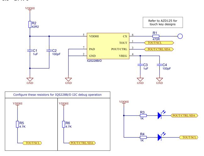
Figure 3.3: Typical application schematic of IQS228B/D. 100 pF capacitors are optional for added RF immunity. Place all decoupling capacitors (on VDDHI and VREG) as close to the IC as possible.
