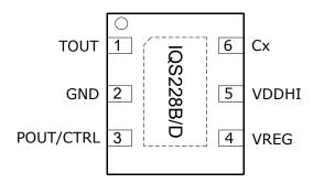
Figure 2.3: IQS228B/D DFN-6 Pin-out
