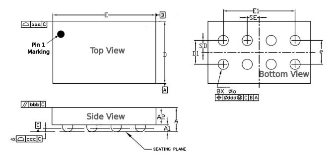
Figure 12.2: IQS228B WLCSP-8 Dimensions (in mm)
