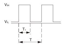
$$V_{\text{IH}} = 4.75 \text{ to } 5.25 \text{ V} \quad V_{\text{IL}} = 0 \text{ to } 0.4 \text{ V}$$
