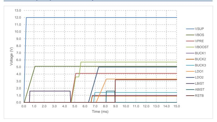
Note: VBOS is set at 5.1 V and RSTB at 3.2 V or 4.9 V to differentiate from regulators on the graph
