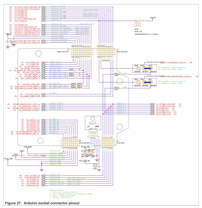
To allow for the flexibility in the design, some of signals on the I/O headers can be swapped for other connections using zero-ohm resistors or jumpers. <u>Table 21</u> describes such signals.
