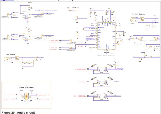
An external DMIC connector is also provided to allow for connecting expansion DMIC boards to the board. This header is shown in <u>Figure 20</u>. Care should be taken when connecting any expansion board with this connector as the supply voltage of ports P0 and P4 should match the necessary supply voltage of the external expansion board.
