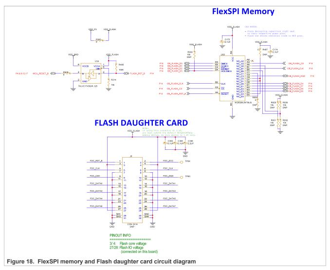
Some of the FlexSPI signals are also multiplexed with the SAI signals for the M.2 connector. Zero-ohm onboard resistors are used to allow the selection of signals either for the QSPI flash memory or for the other connectors (flash data card connector or SAI interface of the M.2 connector). By default, signals for the QSPI flash memory are selected.
