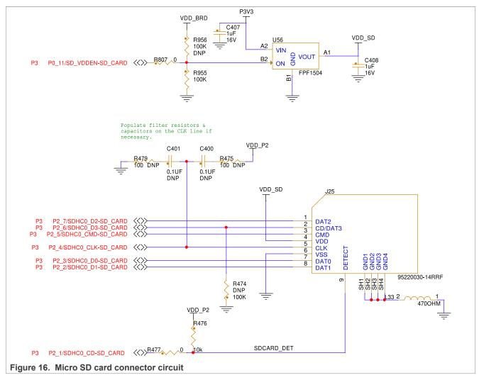
The Port P2\_[7:1] lines that are used for SDHC interface signals are also shared with the M.2 connector (J12) signals and the PWM signals on the Arduino compatible header (J3). Zero-ohm onboard resistors are used to allow the selection of signals between the SDHC card slot or the M.2 connector. The Arduino-compatible header sockets are connected by default, however, can also be disconnected easily by removing the appropriate zero-ohm resistors.
