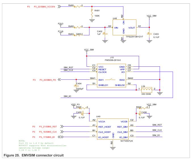
The EMVSIM connector (J10) is supported by a power switch (U48) and a voltage translator (U49). The voltage translator is required to translate the 1.8 V signals from the P3 port to the 3.3 V signals required by the EMVSIM smart cards.
