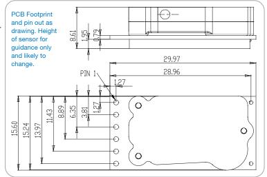
All dimensions in millimeters (mm)
