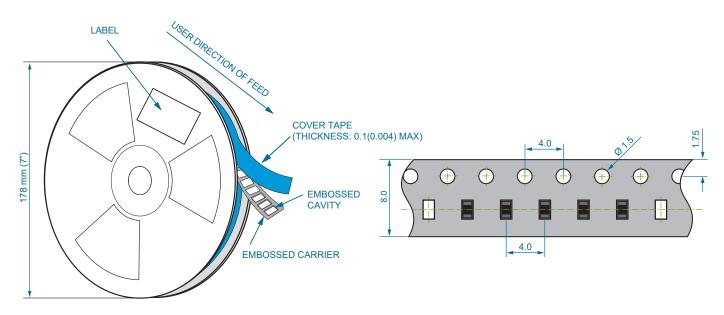
Taping specification: EIA -481 Compliant
