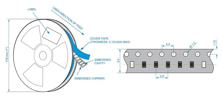
Taping specification: EIA -481 Compliant
