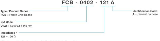
$^{\ast}$  Note: Expressed by three figures. The unit is ohm (Ω). The first and second figures are significant digits, the third figure expresses the number of zeros which follow the two figures.
