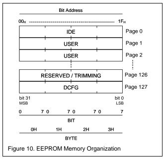
Page 0 holds the device Identifier, IDE, page 126 is reserved and page 127 holds device configuration data (DCFG). Both are programmed during device manufacturing and locked against overwriting, according to section 15. Pages 1 to 126 are available for user data storage.
