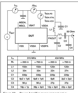
Figure 53. Power Amplifier measurement setup
