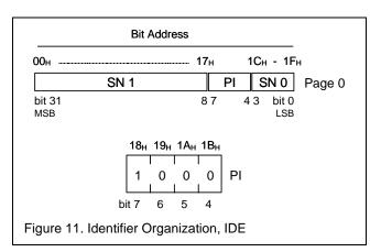
The Identifier is typically employed in the process rolling code or challenge response generation for keyless entry applications. The use of the factory supplied Identifier is not mandatory, instead the device can be configured (DCFG) to employ a 32 bit pattern located in any page in the range 0 to 126.
