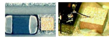
Our ceramic mounting shorts are excellent replacements for kovar and moly-tabs. These ceramic shorts have a much sharper edge and are flat stable bases for mounting semiconductors.
