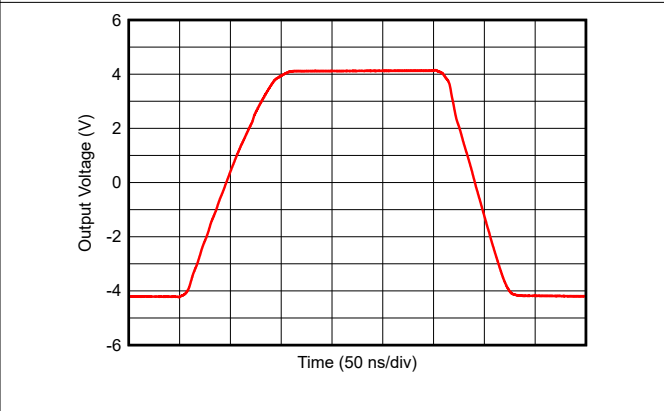
Figure 7-12. Large-Signal Transient Response
