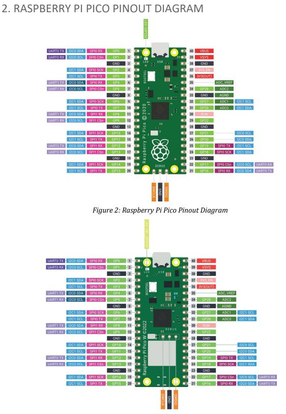
Figure 3: Raspberry Pi Pico W Pinout Diagram
