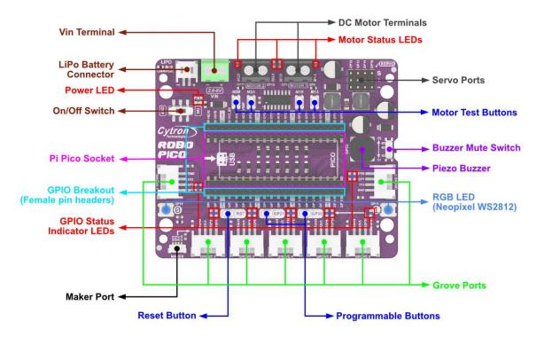
Figure 1: ROBO-PICO Board Functions
