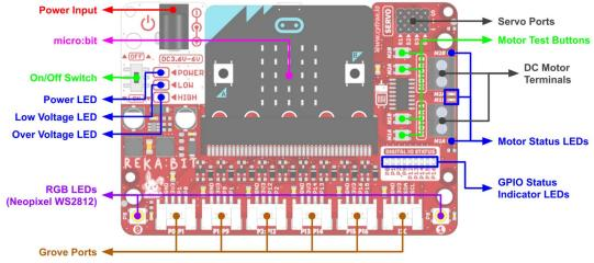
Figure 1: REKA:BIT Board Functions
