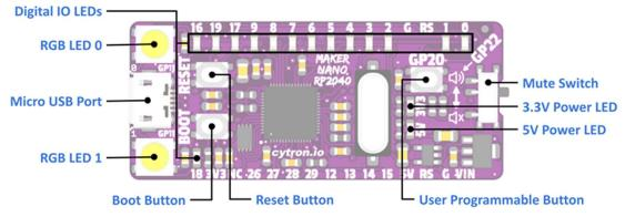
Figure 1: MAKER-NANO-RP2040 Board Functions (Top)
