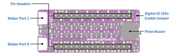
Figure 2: MAKER-NANO-RP2040 Board Functions (Bottom)
