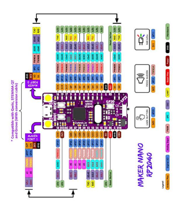
Figure 3: MAKER-NANO-RP2040 Pinout Diagram
