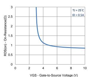
3. On-Resistance vs. Gate-to-Source Voltage
