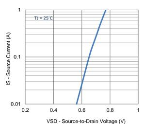
4. Drain-to-Source Forward Voltage
