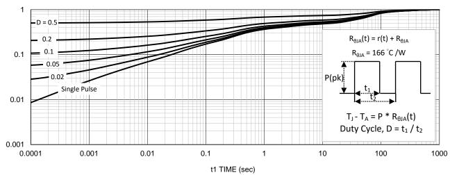
11. Normalized Thermal Transient Junction to Ambient
