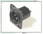
ACM 3 Pin chassis mounting Male XLR with counter sunk mounting holes for M3 screw fixing. XACM has non counter sunk mounting holes for self-tap screw fixing. Nickel Silver plated Brass contacts.
