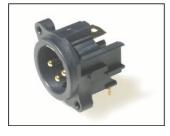
XNACM5 / PC90 3 Pin horizontal PCB mounting male XLR for self-tap screw fixing. Gold plated Brass contacts. Vertical PCB mounting also available, part XNACM5 / PCS
