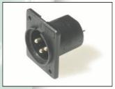
XACM / PCS 3 Pin vertical PCB mounting Male XLR with non counter sunk mounting holes for self-tap screw fixing. ACM PCS has counter sunk mounting holes for M3 screw fixing. Nickel Silver plated Brass contacts.
