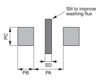
Olt is recommended to provide a slit (about 1mm width) in the board under the components to improve washing flux.
