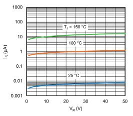
Fig. 4 - Typical Reverse Leakage Current vs. Reverse Voltage
