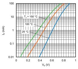
Fig. 1 - Typical Forward Current vs. Forward Voltage
