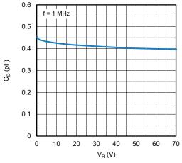
Fig. 3 - Typical Capacitance vs. Reverse Voltage
