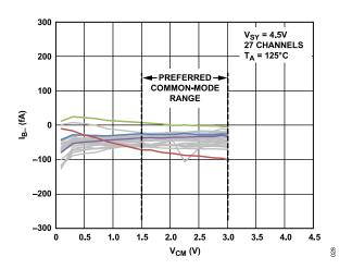
Figure 28. Inverting Input Bias Current ( $I_{B-}$ ) vs. Common-Mode Voltage ( $V_{CM}$ ),  $V_{SY}$  = 4.5 V,  $T_A$  = 125°C
