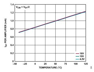
Figure 53. Supply Current (ISY) per Amplifier vs. Temperature
