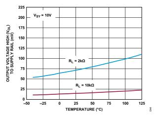
Figure 47. Output Voltage Low ( $V_{OL}$ ) to Supply Rail vs. Temperature,  $V_{SY} = 10$
