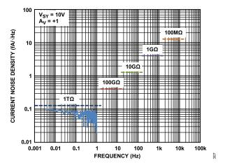
Figure 118. Current Noise Spectral Density
