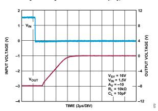
Figure 72. Negative Overload Recovery, V<sub>SY</sub> = 16 V
