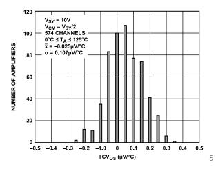
Figure 14. Input Offset Voltage Drift Distribution,  $0^{\circ}C \le T_A \le 125^{\circ}C$ ,  $V_{SY} = 10 \text{ V}$
