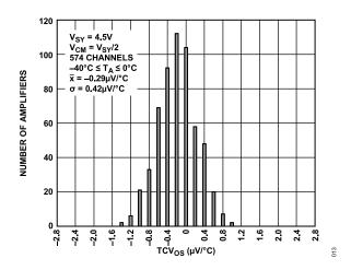
Figure 10. Input Offset Voltage Drift Distribution,  $-40^{\circ}\text{C} \le T_{A} \le 0^{\circ}\text{C}$ ,  $V_{\text{SY}} = 4.5$
