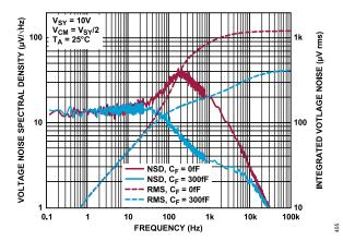
Figure 131. RTO Noise Spectral Density (25°C)
