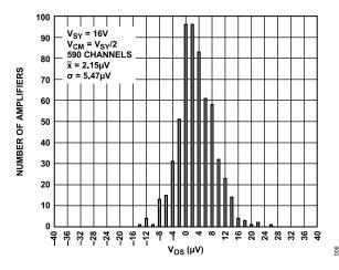
Figure 6. Input Offset Voltage Distribution, V<sub>SY</sub> = 16 V
