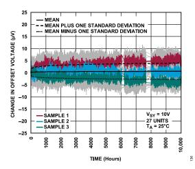
Figure 136. Measured Long-Term Drift of the ADA4530-1 Offset Voltage over 10,000 Hours
