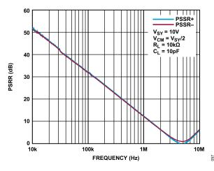
Figure 57. PSRR vs. Frequency
