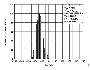
Figure 38. Noninverting Input Bias Current Histogram, T<sub>A</sub> = 125°C, V<sub>SY</sub> = 10 V
