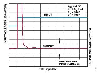
Figure 76. Positive Settling Time to 0.1%,  $V_{SY} = 4.5 \text{ V}$
