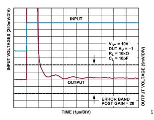
Figure 77. Positive Settling Time to 0.1%,  $V_{SY} = 10 \text{ V}$
