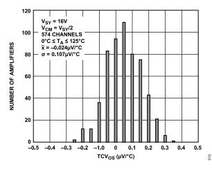
Figure 15. Input Offset Voltage Drift Distribution,  $0^{\circ}C \le T_A \le 125^{\circ}C$ ,  $V_{SY} = 16 \text{ V}$
