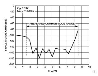
Figure 21. Small Signal CMRR vs. Common-Mode Voltage (V<sub>CM</sub>)
