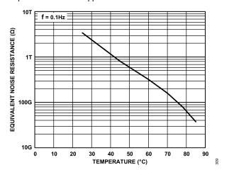
Figure 120. Equivalent Noise Resistance vs. Temperature
