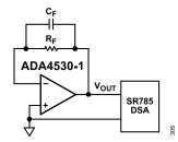
Figure 116. Current Noise Measurement Setup
