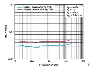
Figure 79. THD + N vs. Frequency,  $V_{SY} = 4.5 \text{ V}$
