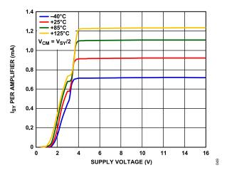
Figure 52. Supply Current (ISY) per Amplifier vs. Supply Voltage (VSY)
