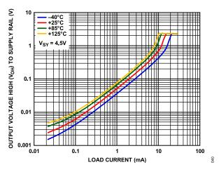
Figure 43. Output Voltage High (V<sub>OH</sub>) to Supply Rail vs. Load Current (I<sub>LOAD</sub>),  $\rm V_{SY}$  = 4.5 V
