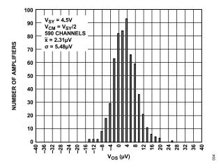
Figure 4. Input Offset Voltage Distribution, V<sub>SY</sub> = 4.5 V
