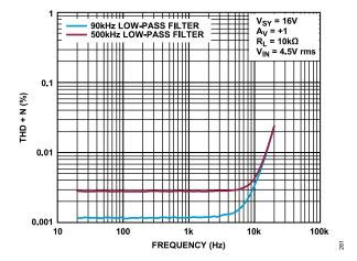
Figure 81. THD + N vs. Frequency,  $V_{SY} = 16 \text{ V}$
