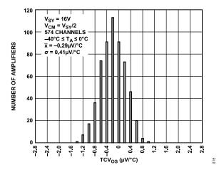
Figure 12. Input Offset Voltage Drift Distribution,  $-40^{\circ}\text{C} \le T_A \le 0^{\circ}\text{C}$ ,  $V_{\text{SY}} = 16 \text{ V}$
