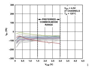
Figure 31. Noninverting Input Bias Current ( $I_{B+}$ ) vs. Common-Mode Voltage ( $V_{CM}$ ),  $V_{SY}$  = 4.5 V,  $T_A$  = 125°C
