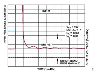
Figure 78. Positive Settling Time to 0.1%,  $V_{SY} = 16 \text{ V}$
