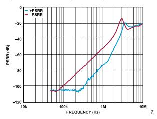
Figure 134. Positive and Negative PSRR for the ADP7118 and ADP7182 Powering ADA4530-1,  $\pm V_{SY} = \pm 5 \text{ V}$ ,  $\pm IN = 0 \text{ V}$
