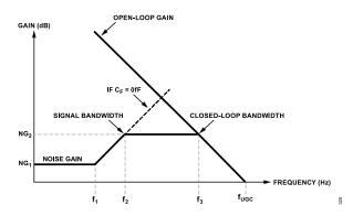
Figure 126. Transimpedance Noise Gain vs. Frequency
