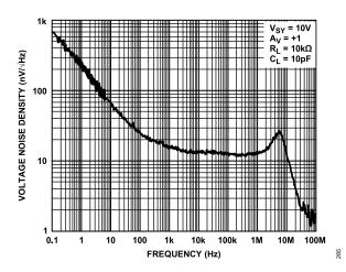
Figure 85. Voltage Noise Density vs. Frequency,  $V_{SY}$  = 10 V
