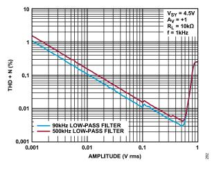
Figure 82. THD + N vs. Amplitude,  $V_{SY} = 4.5 \text{ V}$
