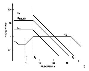
Figure 127. Photodiode TIA RTO Noise Spectral Density
