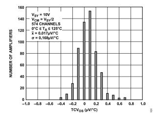
Figure 97. Input Offset Voltage Drift Distribution,  $0^{\circ}C \le T_A \le 125^{\circ}C$ ,  $V_{SY} = 10 \text{ V}$
