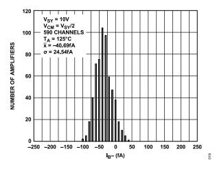
Figure 37. Inverting Input Bias Current Histogram, T<sub>A</sub> = 125°C, V<sub>SY</sub> = 10 V
