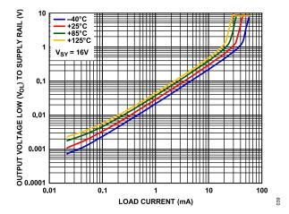
Figure 42. Output Voltage Low  $(V_{OL})$  to Supply Rail vs. Load Current  $(I_{LOAD})$ ,  $V_{SV} = 16 \text{ V}$
