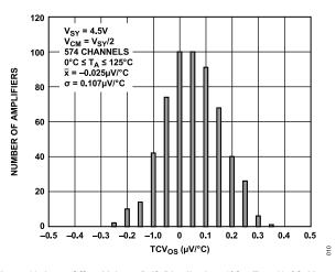
Figure 13. Input Offset Voltage Drift Distribution,  $0^{\circ}\text{C} \le T_{A} \le 125^{\circ}\text{C}$ ,  $V_{\text{SY}} = 4.5$
