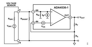
Figure 105. Voltage Buffer Circuit
