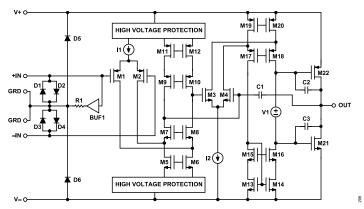
Figure 99. Simplified Schematic
