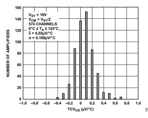
Figure 98. Input Offset Voltage Drift Distribution,  $0^{\circ}C \le T_A \le 125^{\circ}C$ ,  $V_{SY} = 16 \text{ V}$
