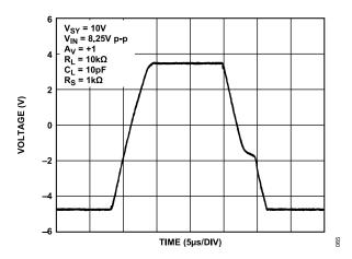
Figure 65. Large Signal Transient Response,  $V_{SY} = 10 \text{ V}$
