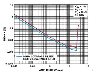
Figure 83. THD + N vs. Amplitude,  $V_{SY} = 10 \text{ V}$
