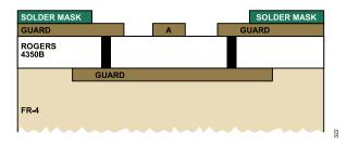
Figure 123. Layout Cross Section with Guard Plane
