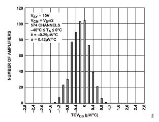
Figure 11. Input Offset Voltage Drift Distribution,  $-40^{\circ}\text{C} \le T_A \le 0^{\circ}\text{C}$ ,  $V_{\text{SY}} = 10 \text{ V}$
