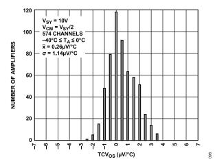
Figure 94. Input Offset Voltage Drift Distribution,  $-40^{\circ}\text{C} \le T_A \le 0^{\circ}\text{C}$ ,  $V_{\text{SY}} = 10 \text{ V}$
