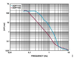
Figure 135. Maximum Allowable Ripple at the Input of the LDOs to Bring Spurs To Noise Floor Level (-120 dB)
