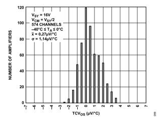
Figure 95. Input Offset Voltage Drift Distribution,  $-40^{\circ}\text{C} \le T_A \le 0^{\circ}\text{C}$ ,  $V_{\text{SY}} = 16 \text{ V}$
