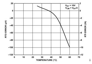
Figure 128. DC Error vs. Temperature
