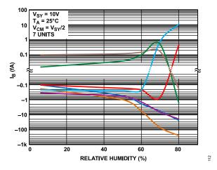
Figure 112. Effective Input Bias Current vs. Relative Humidity
