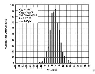
Figure 5. Input Offset Voltage Distribution,  $V_{SY} = 10 \text{ V}$
