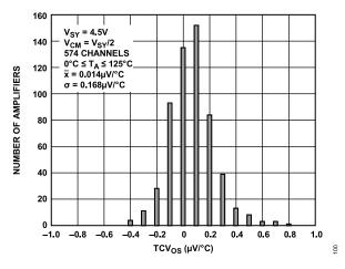
Figure 96. Input Offset Voltage Drift Distribution,  $0^{\circ}\text{C} \le T_A \le 125^{\circ}\text{C}$ ,  $V_{\text{SY}} = 4.5$
