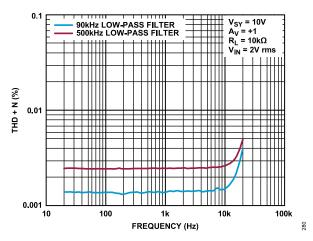
Figure 80. THD + N vs. Frequency, V<sub>SY</sub> = 10 V
