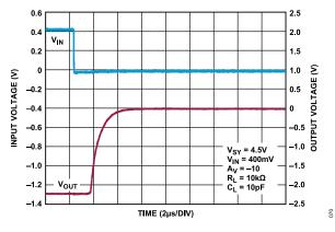
Figure 70. Negative Overload Recovery, V<sub>SY</sub> = 4.5 V
