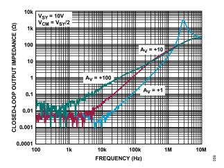
Figure 59. Closed-Loop Output Impedance vs. Frequency
