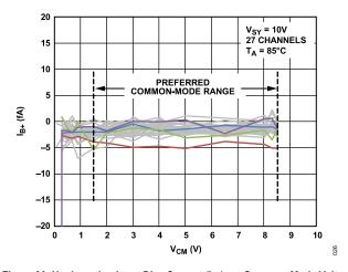
Figure 26. Noninverting Input Bias Current ( $I_{B+}$ ) vs. Common-Mode Voltage ( $V_{CM}$ ),  $V_{SY}$  = 10 V,  $T_A$  = 85°C
