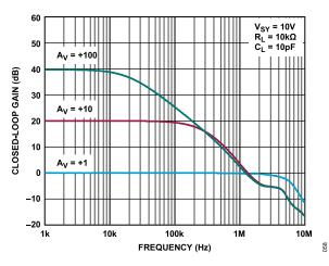
Figure 58. Closed-Loop Gain vs. Frequency
