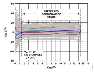
Figure 18. Input Offset Voltage ( $V_{OS}$ ) vs. Common-Mode Voltage ( $V_{CM}$ ),  $V_{SY}$  = 16 V
