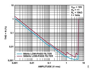
Figure 84. THD + N vs. Amplitude,  $V_{SY} = 16 \text{ V}$
