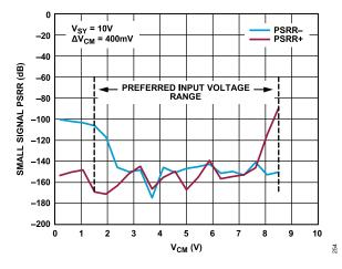
Figure 54. Small Signal PSRR vs. Common-Mode Voltage (V<sub>CM</sub>)
