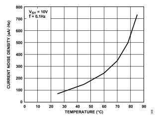
Figure 119. Current Noise Density vs. Temperature
