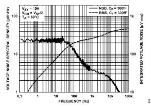
Figure 132. RTO Noise Spectral Density (60°C)
