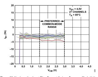
Figure 25. Noninverting Input Bias Current ( $I_{B+}$ ) vs. Common-Mode Voltage ( $V_{CM}$ ),  $V_{SY}$  = 4.5 V,  $T_A$  = 85°C
