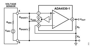
Figure 107. Voltage Buffer Circuit with Guard
