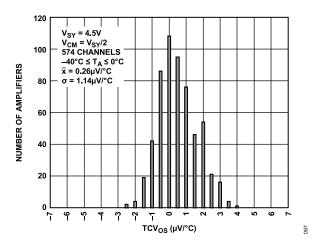
Figure 93. Input Offset Voltage Drift Distribution,  $-40^{\circ}\text{C} \le T_A \le 0^{\circ}\text{C}$ ,  $V_{\text{SY}} = 4.5$
