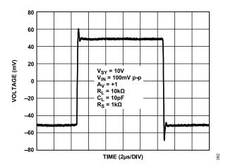
Figure 62. Small Signal Transient Response, V<sub>SY</sub> = 10 V
