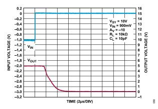
Figure 68. Positive Overload Recovery, V<sub>SY</sub> = 10 V
