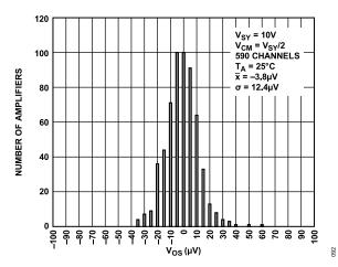
Figure 88. Input Offset Voltage Distribution,  $V_{SY} = 10 \text{ V}$
