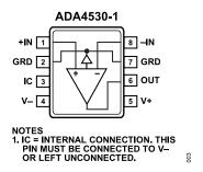
Figure 3. Pin Configuration
