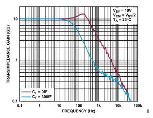
Figure 129. Transimpedance Gain vs. Frequency
