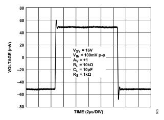
Figure 63. Small Signal Transient Response,  $V_{SY} = 16 \text{ V}$
