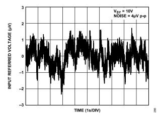
Figure 86. 0.1 Hz to 10 Hz Noise
