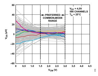
Figure 16. Input Offset Voltage ( $V_{OS}$ ) vs. Common-Mode Voltage ( $V_{CM}$ ),  $V_{SY}$  = 4.5 V
