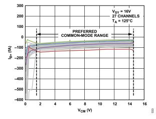
Figure 33. Noninverting Input Bias Current ( $I_{B+}$ ) vs. Common-Mode Voltage ( $V_{CM}$ ),  $V_{SY}$  = 16 V,  $T_A$  = 125°C
