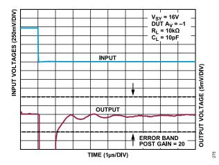
Figure 75. Negative Settling Time to 0.1%,  $V_{SY} = 16 \text{ V}$
