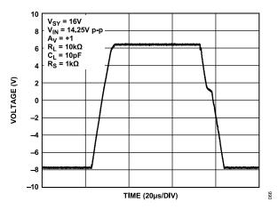
Figure 66. Large Signal Transient Response, V<sub>SY</sub> = 16 V
