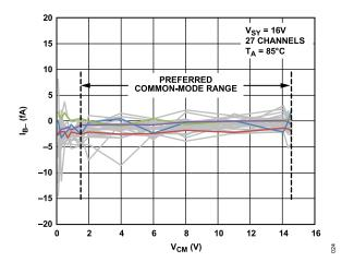
Figure 24. Inverting Input Bias Current ( $I_{B-}$ ) vs. Common-Mode Voltage ( $V_{CM}$ ),  $V_{SY} = 16 \text{ V}$ ,  $T_A = 85^{\circ}\text{C}$
