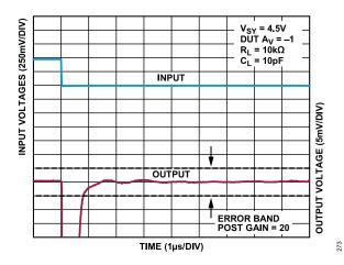
Figure 73. Negative Settling Time to 0.1%, V<sub>SY</sub> = 4.5 V
