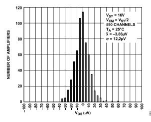
Figure 89. Input Offset Voltage Distribution, V<sub>SY</sub> = 16 V
