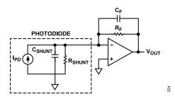
Figure 125. Transimpedance Amplifier with Photodiode Model
