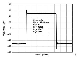
Figure 61. Small Signal Transient Response, V<sub>SY</sub> = 4.5 V
