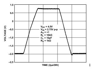
Figure 64. Large Signal Transient Response,  $V_{SY} = 4.5 \text{ V}$
