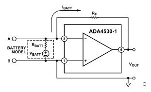
Figure 115. TIA Circuit with Contamination Battery
