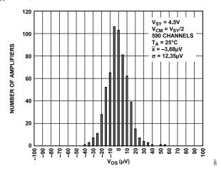
Figure 87. Input Offset Voltage Distribution, V<sub>SY</sub> = 4.5 V
