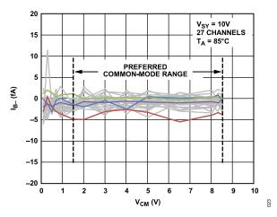
Figure 23. Inverting Input Bias Current ( $I_{B-}$ ) vs. Common-Mode Voltage ( $V_{CM}$ ),  $V_{SY} = 10 \text{ V}$ ,  $T_A = 85^{\circ}\text{C}$
