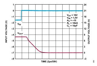
Figure 69. Positive Overload Recovery,  $V_{SY}$  = 16 V
