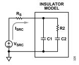
Figure 108. Dielectric Relaxation Model Test Circuit
