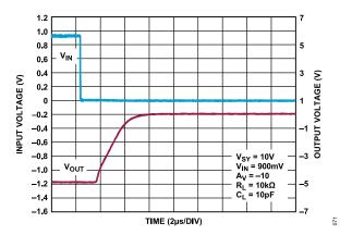
Figure 71. Negative Overload Recovery, V<sub>SY</sub> = 10 V
