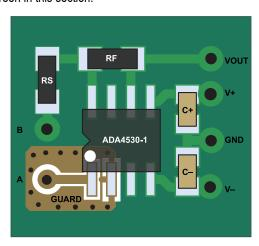
Figure 121. Buffer Circuit Layout
