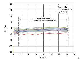
Figure 27. Noninverting Input Bias Current ( $I_{B+}$ ) vs. Common-Mode Voltage ( $V_{CM}$ ),  $V_{SY}$  = 16 V,  $T_A$  = 85°C
