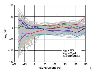
Figure 92. Input Offset Voltage ( $V_{OS}$ ) vs. Temperature,  $V_{SY}$  = 16 V
