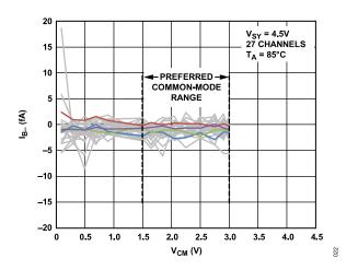
Figure 22. Inverting Input Bias Current (I<sub>B</sub>-) vs. Common-Mode Voltage ( $V_{CM}$ ),  $V_{SY}$  = 4.5 V,  $T_A$  = 85°C
