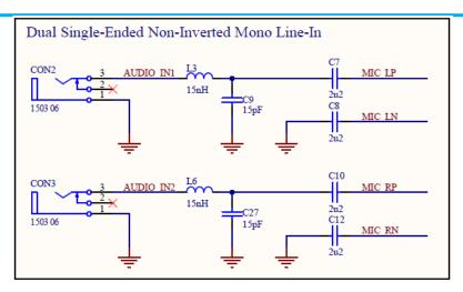
One 2-pole audio jack providing single mono audio source, unused inputs are AC grounded
