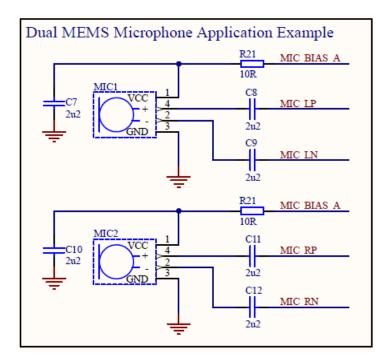
If a single microphone is used, the unused analogue inputs should be AC coupled to ground.
