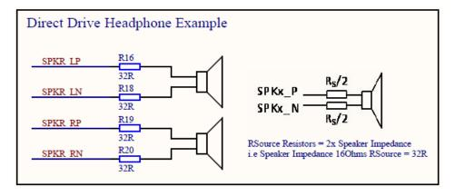
To achieve optimal audio performance in direct drive applications the DACs should operate at close the maximum output voltage of 1Vrms. This can be achieved by adding source resistors between the output terminals and the speaker driver, the value of which are double the rated speaker impedance. i.e., for 16 $\Omega$  speakers use 32 $\Omega$  resistors, for 32 $\Omega$  speakers use 64 $\Omega$  resistors.
