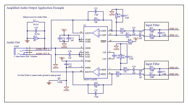
Some amplifiers do not support "capless" operation and require ac coupling on the input and output of the amplifier. Series capacitance can introduce clicks and pops during turn off and turn on as voltage transients occur across the capacitors causing audible spikes on the audio output.
