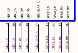
All analogue inputs are DC coupled and must be externally ac coupled for correct operation.
