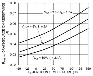
Figure 7. On-Resistance Variation with Temperature
