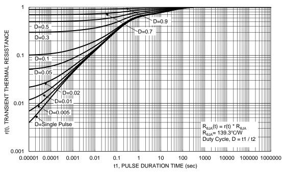
Figure 13. Transient Thermal Resistance
