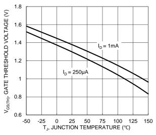
Figure 8. Gate Threshold Variation vs. JunctionTemperature
