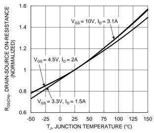
Figure 6. On-Resistance Variation with Temperature
