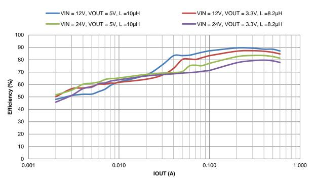
Figure 2. AP64060 Efficiency vs. Output Current
