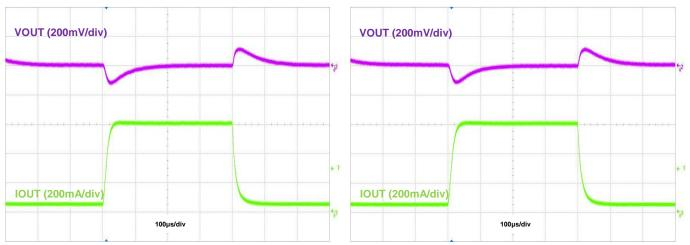
Figure 18. Load Transient, VIN = 12V, IOUT = 50mA to 600mA
