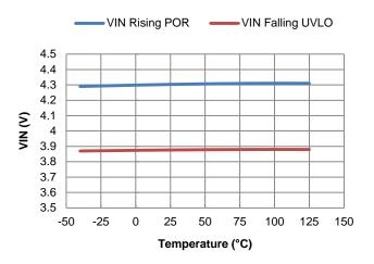
Figure 12. VIN Power-On Reset and UVLO vs. Temperature
