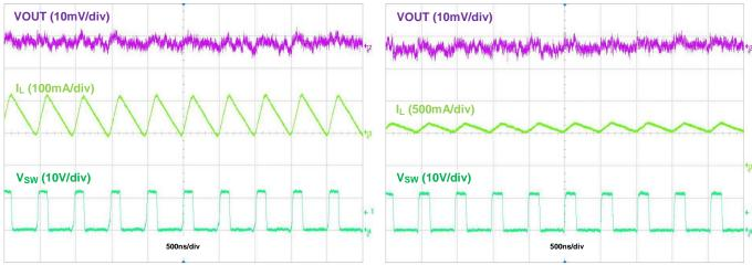
Figure 16. Output Voltage Ripple, VOUT = 3.3V; IOUT = 50mA
