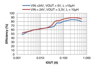
Figure 4. Efficiency vs. Output Current, VIN = 12V
