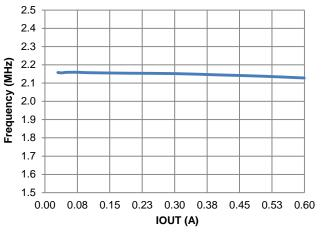
Figure 13. f<sub>SW</sub> vs. IOUT (A)
