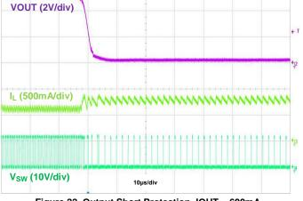
Figure 22. Output Short Protection, IOUT = 600mA
