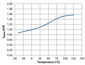
Figure 11. I<sub>SHDN</sub> vs. Temperature
