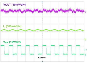
Figure 15. Output Voltage Ripple, VOUT = 5V; IOUT = 600mA
