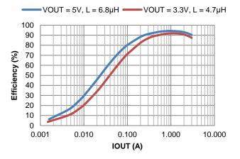
Figure 26. Efficiency vs. Output Current, VIN = 12V
