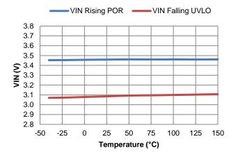
Figure 8. VIN Power-On Reset and UVLO vs. Temperature
