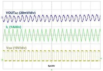
Figure 20. Output Voltage Ripple, VOUT = 5V, IOUT = 3A
