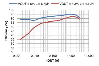
Figure 13. Efficiency vs. Output Current, VIN = 12V
