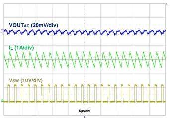
Figure 36. Output Voltage Ripple, VOUT = 3.3V, IOUT = 3A
