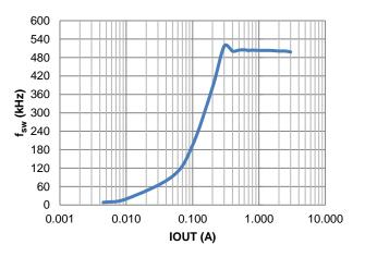
Figure 18. fsw vs. Load
