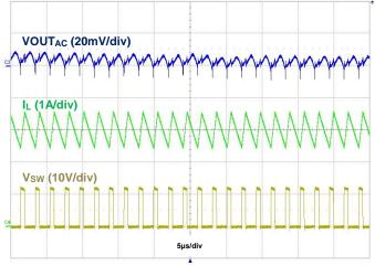
Figure 22. Output Voltage Ripple, VOUT = 3.3V, IOUT = 3A
