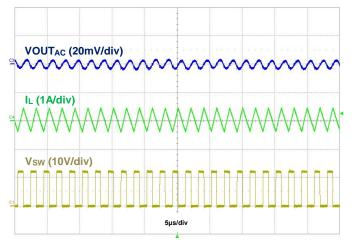
Figure 33. Output Voltage Ripple, VOUT = 5V, IOUT = 50mA
