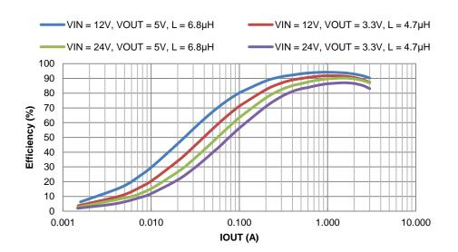
Figure 3. Efficiency vs. Output Current, AP63301Q
