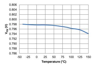
Figure 6. Feedback Voltage vs. Temperature, IOUT = 1A
