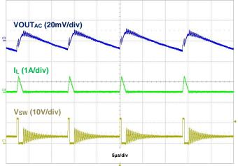
Figure 21. Output Voltage Ripple, VOUT = 3.3V, IOUT = 50mA
