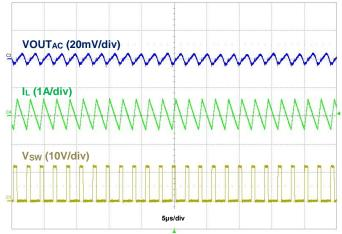
Figure 35. Output Voltage Ripple, VOUT = 3.3V, IOUT = 50mA
