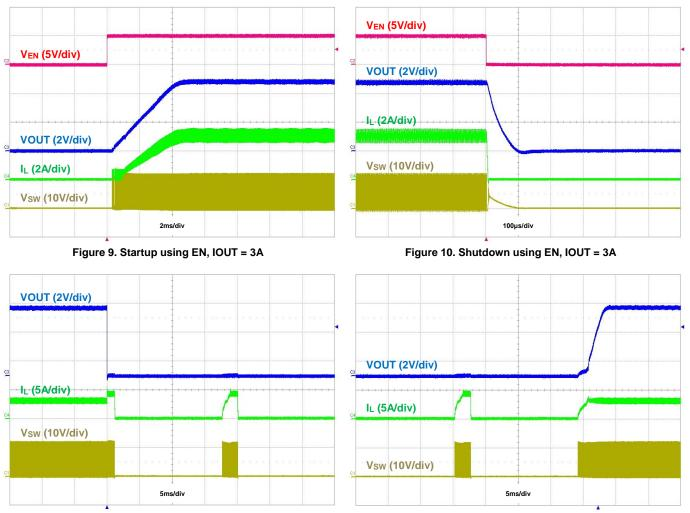
Figure 11. Output Short Protection, IOUT = 3A
