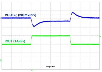
Figure 37. Load Transient, IOUT = 50mA to 500mA to 50mA
