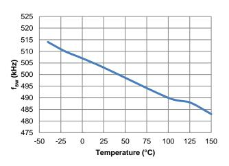
Figure 31. fsw vs. Temperature, IOUT = 0A
