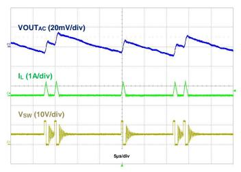
Figure 19. Output Voltage Ripple, VOUT = 5V, IOUT = 50mA
