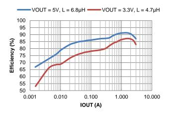
Figure 14. Efficiency vs. Output Current, VIN = 24V
