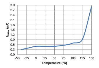
Figure 7. ISHDN vs. Temperature
