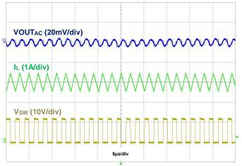
Figure 34. Output Voltage Ripple, VOUT = 5V, IOUT = 3A
