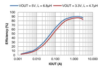
Figure 27. Efficiency vs. Output Current, VIN = 24V
