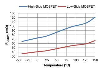
Figure 5. Power MOSFET RDS(ON) vs. Temperature
