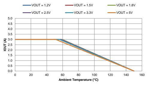
Figure 41. Output Current Derating Curve vs. Ambient Temperature, VIN = 12V
