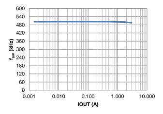
Figure 32. fsw vs. Load
