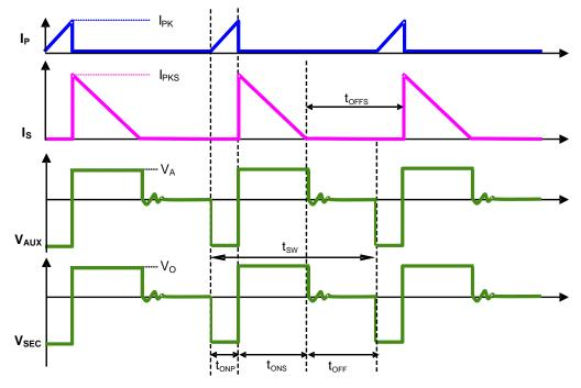
Figure 1. The Operation Waveform of Flyback PSR System
