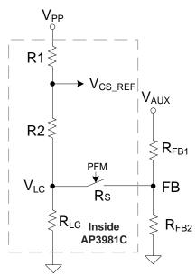
Figure 5. Line Compensation Control Circuit
