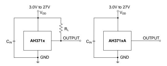
Note: 4. C<sub>IN</sub> is for power stabilization and to strengthen the noise immunity, the recommended capacitance is 10nF to 100nF. R<sub>L</sub> is the pullup resistor.
