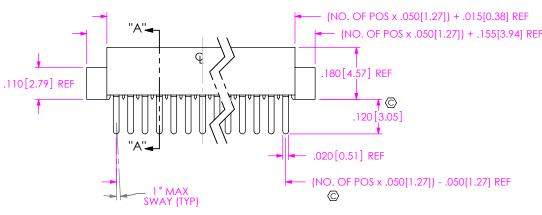
FIG 1 THROUGH HOLE/STRAIGHT MODIFIED
