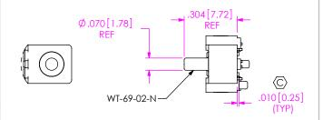
FIG 10 -PP OPTION (SEAF-20-05.0-XX-06-1-A-PP-K-TR SHOWN) (SOME CENTER FEATURES REMOVED FOR CLARITY) (SAME AS FIG 8 EXCEPT AS SHOWN)
