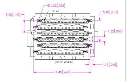
FIG 5 NVAF-DP-06-1-05.0-X-X-K-XR SHOWN (SAME AS FIG 1, EXCEPT AS SHOWN)
