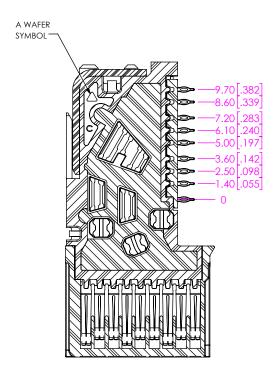
SECTION 'B'-'B' SCALE 3:1 (WAFER A) (HS OR LC OPTIONS)
