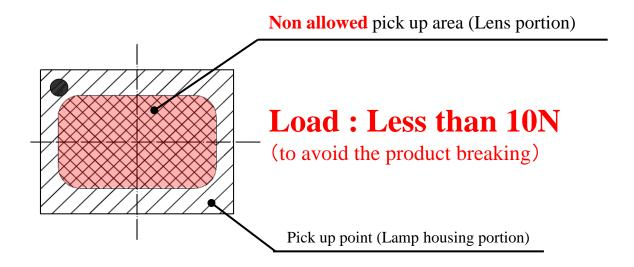
Please adjust the load, the pick up point, the nozzle diameter and etc. before mounting because the over load can cause the breakage of the lamp housing.
