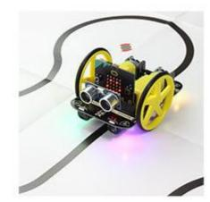
Packed with sensors Integrated Ultrasonic and Line Following sensors for out of the box autonomy
