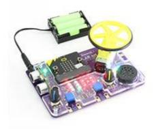
Highly Interactive With 4 onboard inputs and 5 onboard outputs, plus those added by the micro:bit itself.
