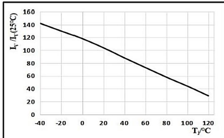
Figure 4. Junction Temperature Vs. Relative Intensity
