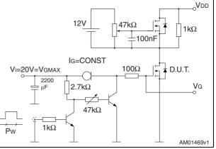
Gate charge test circuit
