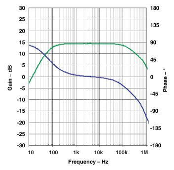
Figure 6. Gain and Phase vs Frequency
