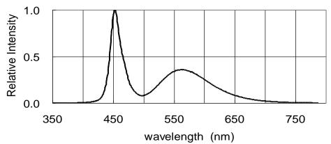
Fig.1 RELATIVE INTENSITY VS. WAVELENGTH
