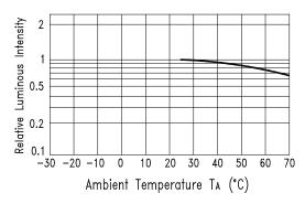
Fig.5 Luminous Intensity vs.
