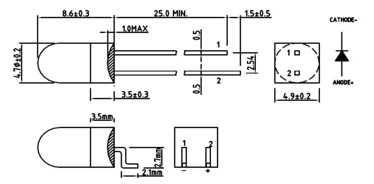
SING: 1. Cathode 2. Anode Tolerance is ±0.25mm unless otherwise specified
